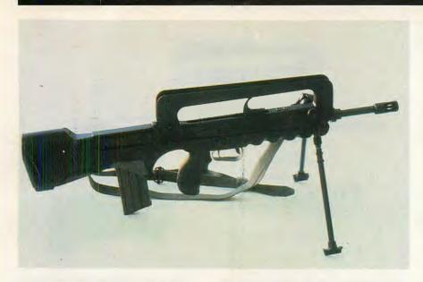
to the barrel and receiver, extends back to the magazine well and cannot be removed. To accommodate the bullpup configuration, the trigger mechanism and pistol grip have been mounted to the lower handguard, forward of the magazine well. The ergonomically-designed pistol grip has three finger grooves and a storage trap which contains a plastic bottle of lubricant.
